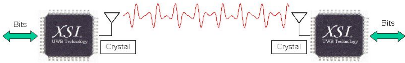
Figure 9: Concept of UWB baseband system implementation
